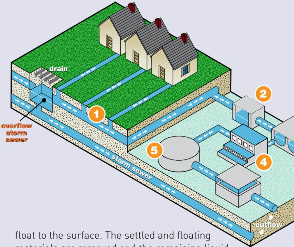
float to the surface. The settled and floating materials are removed and the remaining liquid may be discharged or subjected to further secondary treatment.
